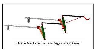
allows the system to aid users in lifting and lowering. When loading a bike, the system holds the rack tray in a lowered position, allowing the user to easily place the bike on the rack and secure it. The Giraffe Rack can accommodate either one or two bikes per vehicle side.
