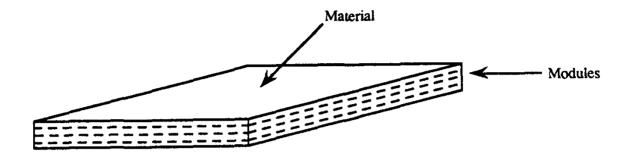
Figure 3.1: Modules in an insulating material
